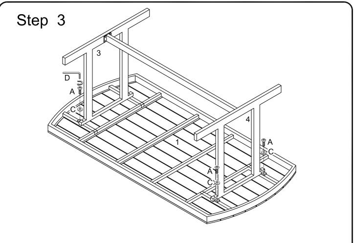
Use wrench (D), bolt (A), washer (C) to secure the side frame (3,4) to the top panel (1).
