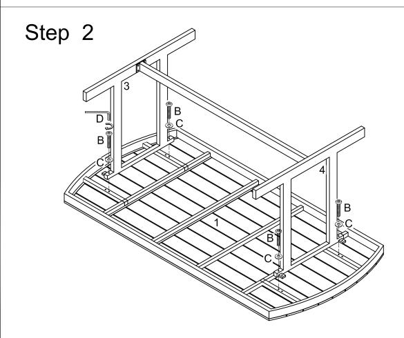
Use wrench (D), bolt (B), washer (C) to secure the side frame (3,4) to the top panel (1).
