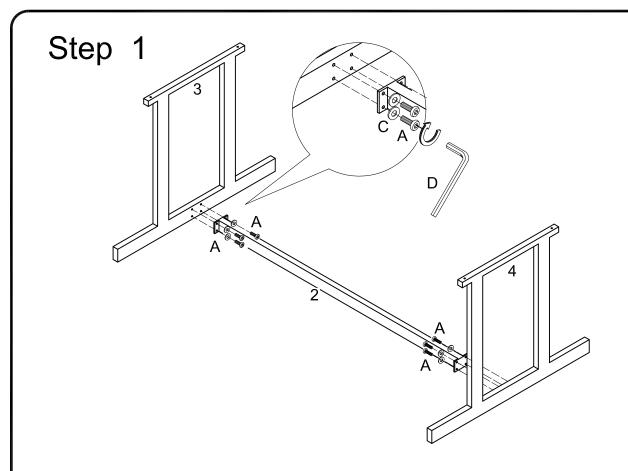
Use wrench (D), bolt (A), washer (C) to secure the cross bar (2) to the side frame (3,4).
